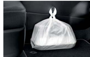
Take away hook. Mounted on the lower passenger side of the centre console, the hook secures bags containing food & drink "to go", to reduce the chance of spillage while on the move. (Reference picture). 99743ADE00
