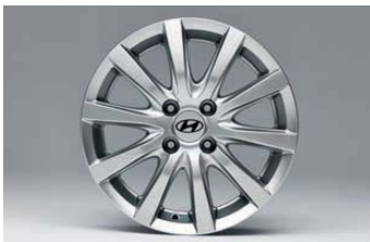
Alloy wheel 15" Halla. 15" ten-spoke alloy wheel, silver, 6.0x15, suitable for 185/65 R15 tyres. CB400ADE01 (TPMS compatible)
