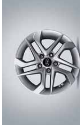
1. Alloy wheel 16" . 16" five-double-spoke alloy wheel, 6.5Jx16, suitable for 215/70 R16 tyres. Not for vehicles with electric parking brake. Cap and nuts not included. 52910D7110PAC
