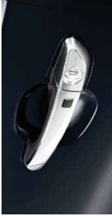
Door handle recess protection foils. Keeps your paintwork looking fresh and new by protecting it from fingernail and other scratches. Made from durable, transparent film. Set of 4. 99272ADE00
